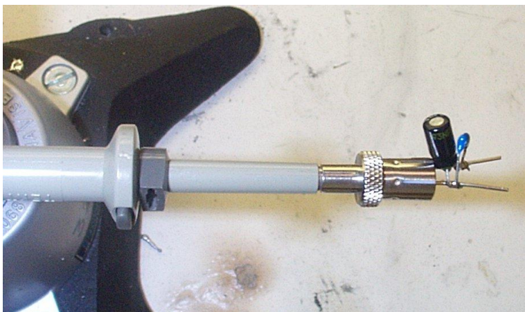
Figure 29 – Oscilloscope Probe with Probe Master 5125BA BNC Adapter (Modified with Wires for Probe Ground for Ripple Measurement, and Two Parallel Decoupling Capacitors Added).
