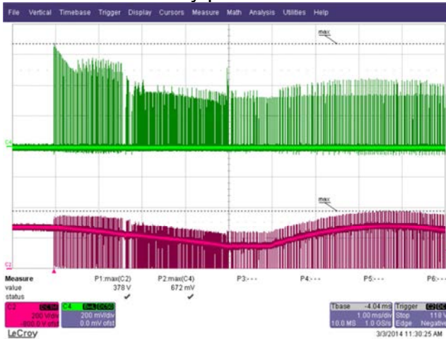
Figure 36 – 190 VAC Input and Maximum Load. Upper: I_{DRAIN} , 0.2 A / div. Lower: V_{DRAIN} , 200 V / div. Time Scale: 1 ms / div.
