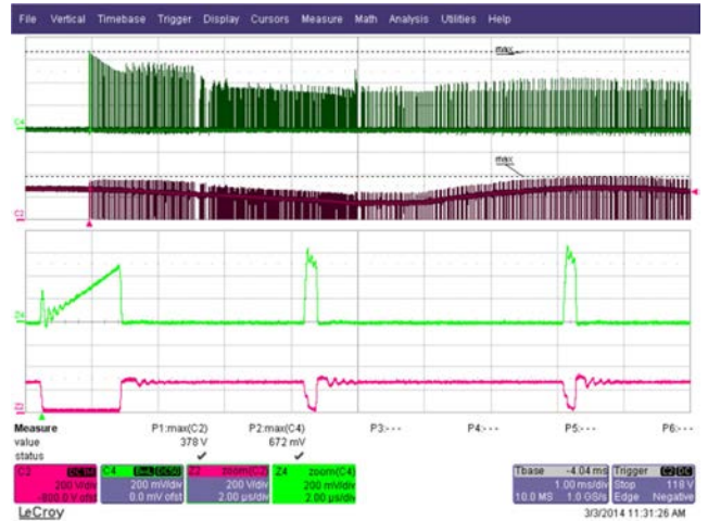
Figure 37 – 190 VAC Input and Maximum Load. Upper: I_{DRAIN} , 0.2 A / div. Lower: V_{DRAIN} , 200 V / div. Time Scale: 1 ms / div. Zoom Time Scale: 2 \mu s / div.
