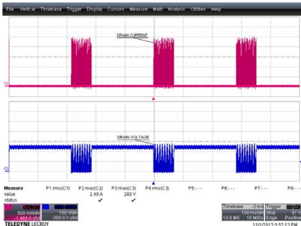
Figure 33 – 185 VAC 50 Hz, Output Short. Upper: I_{DRAIN} , 0.5 A / div. Lower: V_{DRAIN} , 100 V, 100 ms / div.
