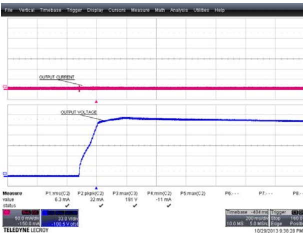
Figure 36 – 230 VAC 50 Hz, Open Load Start-up Upper: I_{OUT} , 50 mA / div. Lower: V_{OUT} , 50 V, 200 ms / div.
