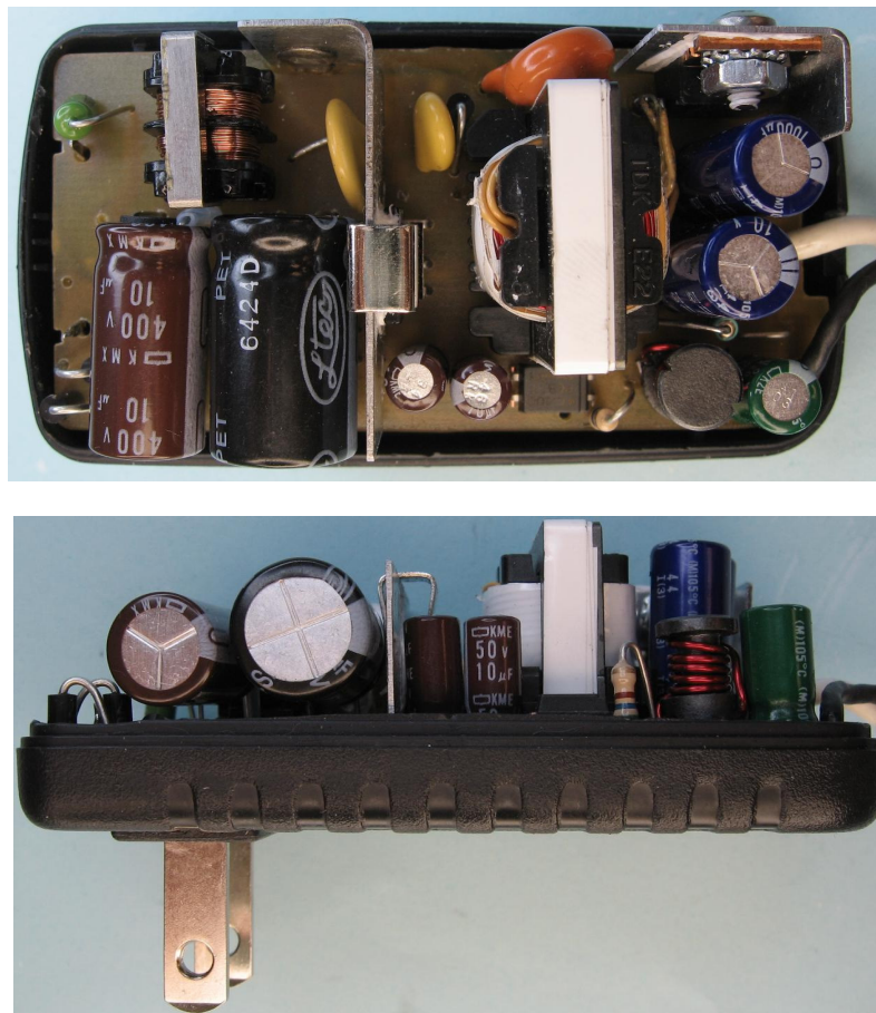
Figure 1 – Populated Circuit Board Photograph.
