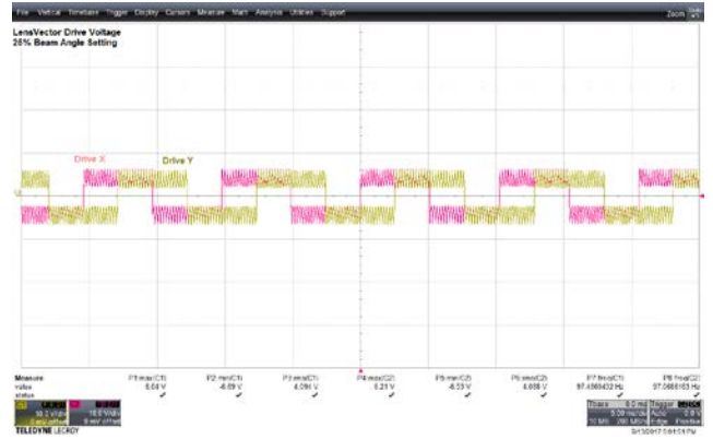
Figure 54 – 120 VAC, 25% Beam Angle Setting.
