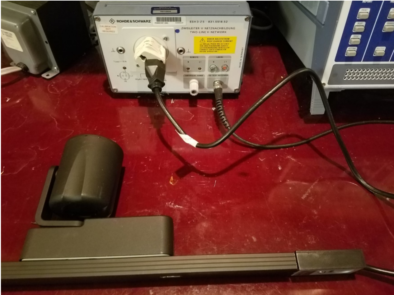
Figure 65 – Conducted EMI Set-up.
