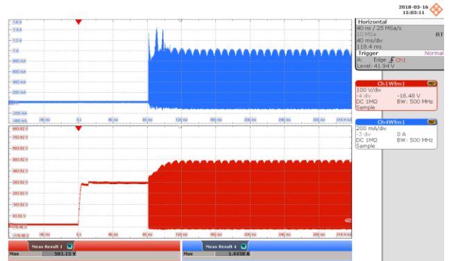
Figure 63 – 265 VAC 50 Hz, Full Load Start-up. Upper: I_{DRAIN} , 200 mA / div. Lower: V_{DRAIN} , 100 V / div., 40 ms / div.
