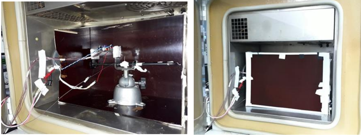
Figure 27 – Test Set-up Pictures. Unit is Placed Inside an Enclosure to Prevent the Effect of Airflow.
