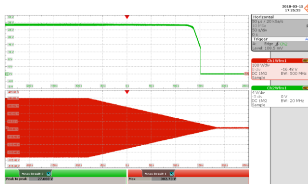
Figure 93 – Brown-out Test at 1 V / s. Ch1: V_{OUT} , 4 V / div. Ch2: V_{IN} , 100 V / div. Time Scale: 50 s / div.
