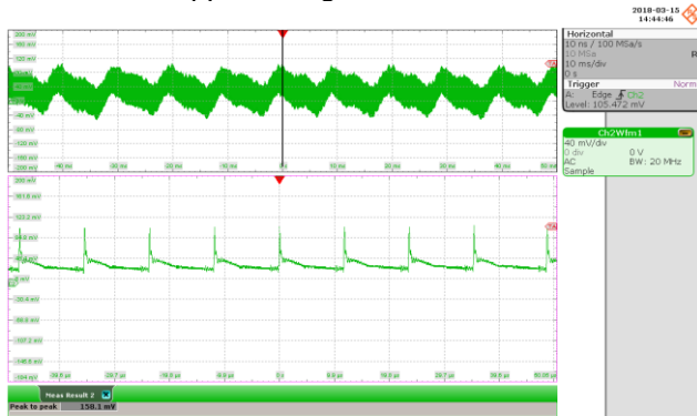
Figure 70 – 230 VAC 50 Hz, Full Load. AC Coupling, 20 MHz Bandwidth. V_{OUT} , 40 mV / div., 10 ms / div. Ripple Voltage: 158.1 mV PK-PK .
